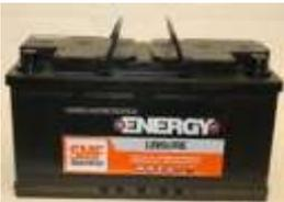
Increasingly, caravan manufacturers are fitting 'maintenance free' or 'sealed for life', These have cells that have no filler caps, and which are not intended to be topped up with water. These batteries must not be overcharged since this will reduce the level of the electrolyte in the cells, which cannot be replenished.
